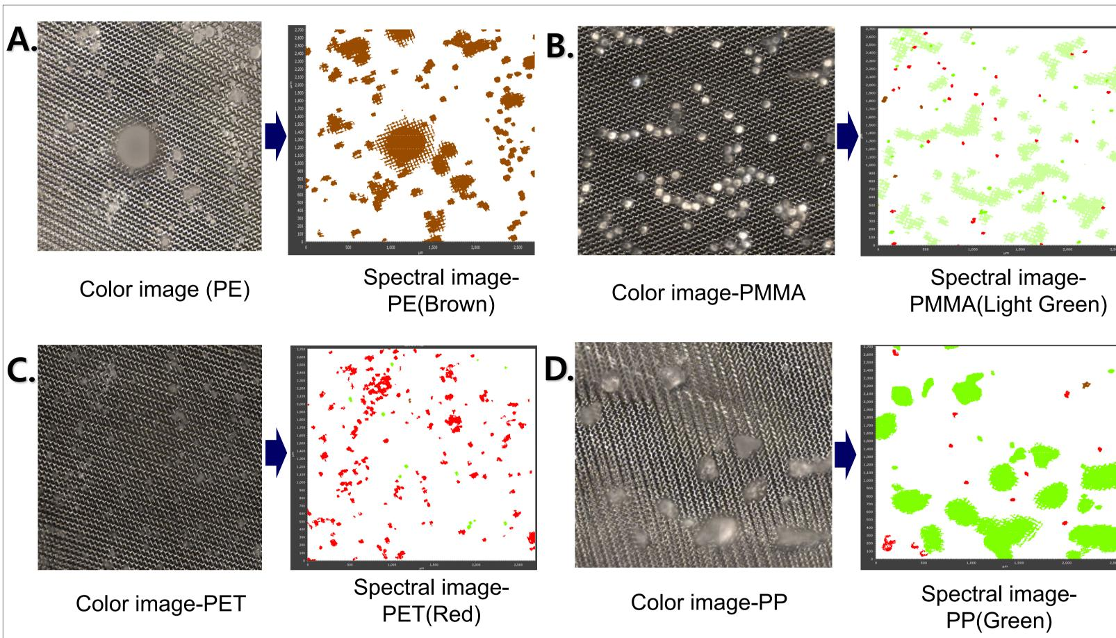
**Figure 1.** Color image of MP and image detected using FT-IR after registration of standard sample(Using siMPle software, Aalborg University, Denmark and Alfred Wegener Institute, Germany); A) PE, B)PMMA, C)PET, D)PP.
