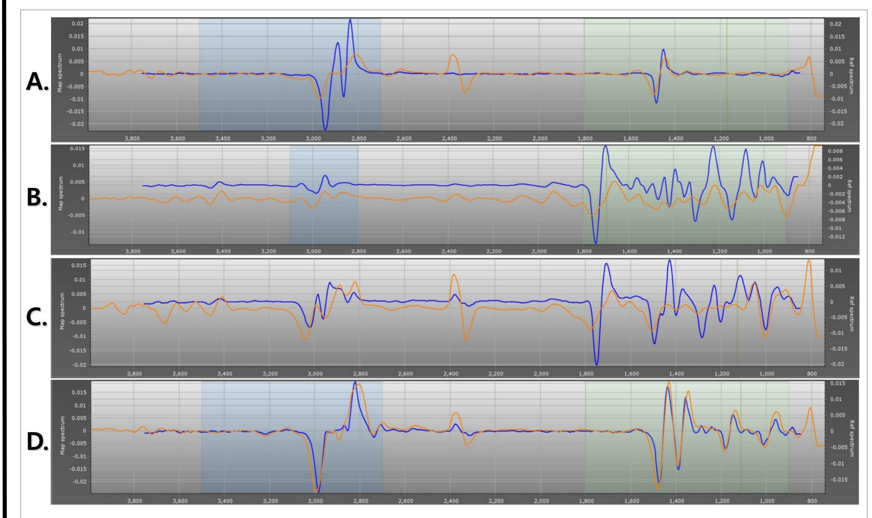
Figure 2. First-order differential graph of FT-IR spectrum; A) PE, B)PMMA, C)PET, D)PP.
