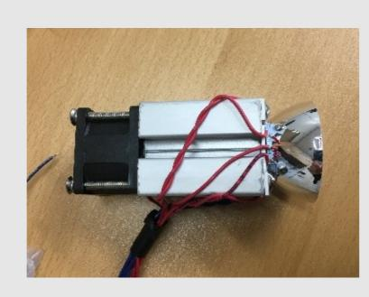
For the full spectral coverage of the TH-lamp, two types of LEDs were used to build the Vis+NIR LED module; GW CSSRM2.EM (OSRAM GmbH, Munich, Germany) and SFH4776, which are a warm-white LED (400–650 nm) and pc-NIR LED(600-1000nm).
