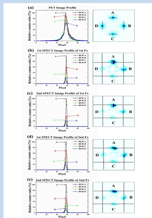
Fig. 3. The image profiles (left column) obtained from four boron uptake regions (BURs) in the reconstructed image with black dotted guidelines (right column).
