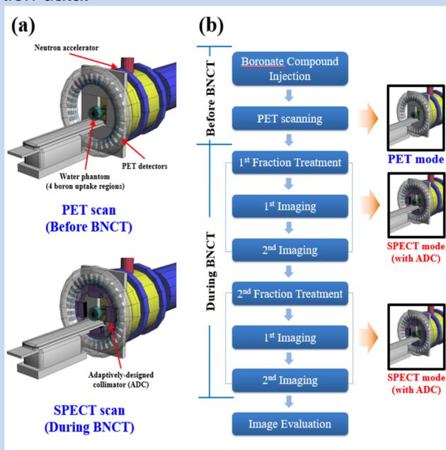
Fig. 1. Simulation configuration of the acquisition of two image types before (top in (a)) and during BNCT (bottom in (a)) and a diagram of the proposed BNCT procedure (b).
