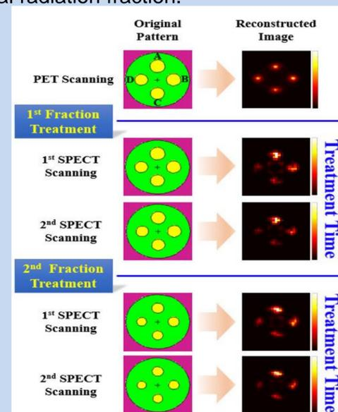
Fig. 2. A diagram of the original patterns and reconstructed images depending on the proposed BNCT procedure.
