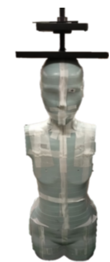
Fig 2. Atom phantom (CIRS, US)
