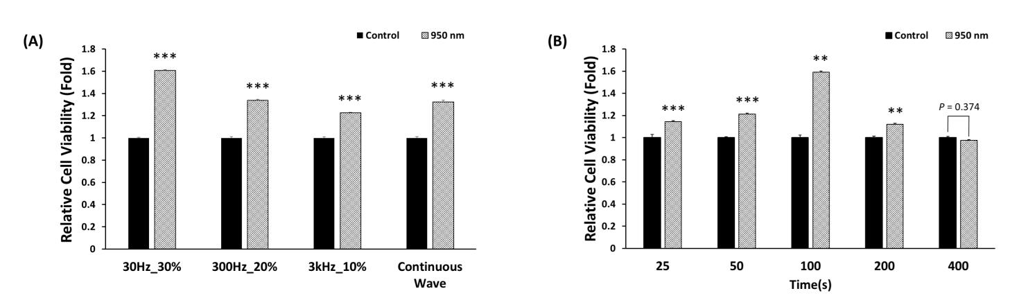
Figure 2. Optimization of 950 nm NIR irradiation conditions for cell viability. (A) Relative cell viability at energy density of 175.68 mJ/cm2. (B) Relative cell viability with different energy densities. Light with the same frequency and duty cycle, 30 Hz and 30%, was applied with different exposure times. Data are mean  $\pm$  standard deviation (SD) (n = 10). \*\*P < 0.01, \*\*\*P < 0.001 versus controls. P values were determined with one-way ANOVA.
